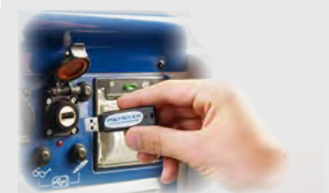
USB memory stick for saving, loading and archiving of welding programs and monitored welding data
