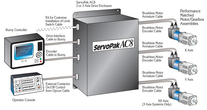
The ServoPak AC8 Servo Drive system delivers the increased power and precision required by competitive production machinery. Integrating user-configurable DSPbased digital drive modules and maintenance-free servo motors, the ServoPak AC8 forms an optimized drive system solution for coordinated motion control. Additional features:
