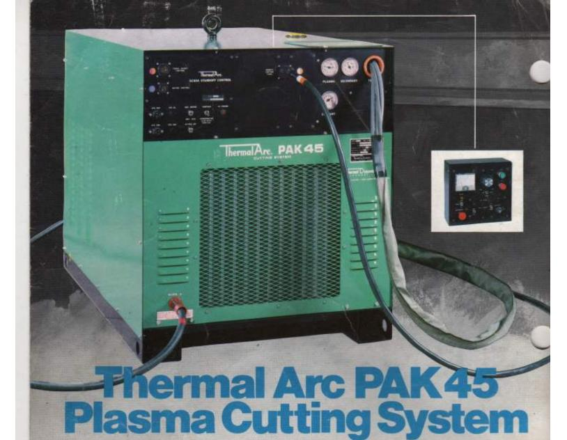
The PAK 45 is a compact, versatile plasma cutting system designed for high speed cutting of most metals up to 2" thick (51 mm), with maximum cutting capability to 3" (76 mm). The cutting current is continuously adjustable between 50 and 400 amperes, to enable quality hand or machine cutting over a wide range of material thicknesses.
