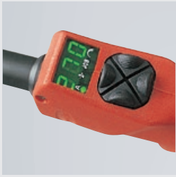
/ JobMaster with integral remote-control functionality
